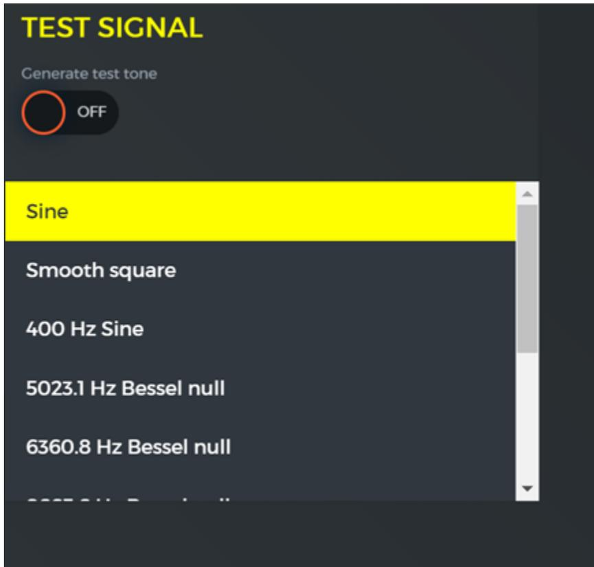
Turning the test generator on will interrupt any feed from the decoder<sub>[GS2]</sub> and place test tones on the output of the chosen sound card. This drop-down menu provides a number of useful test signals to test the linearity of your sound card and the rest of your transmission chain.
