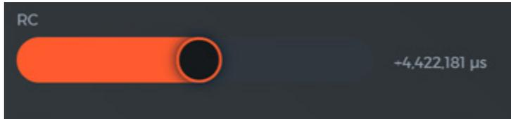
Using the “Smooth Square” signal, adjust the RC slider as necessary to achieve square flat top waveform at frequencies of 30Hz, 400Hz and 10kHz on the test signal generator to the right
