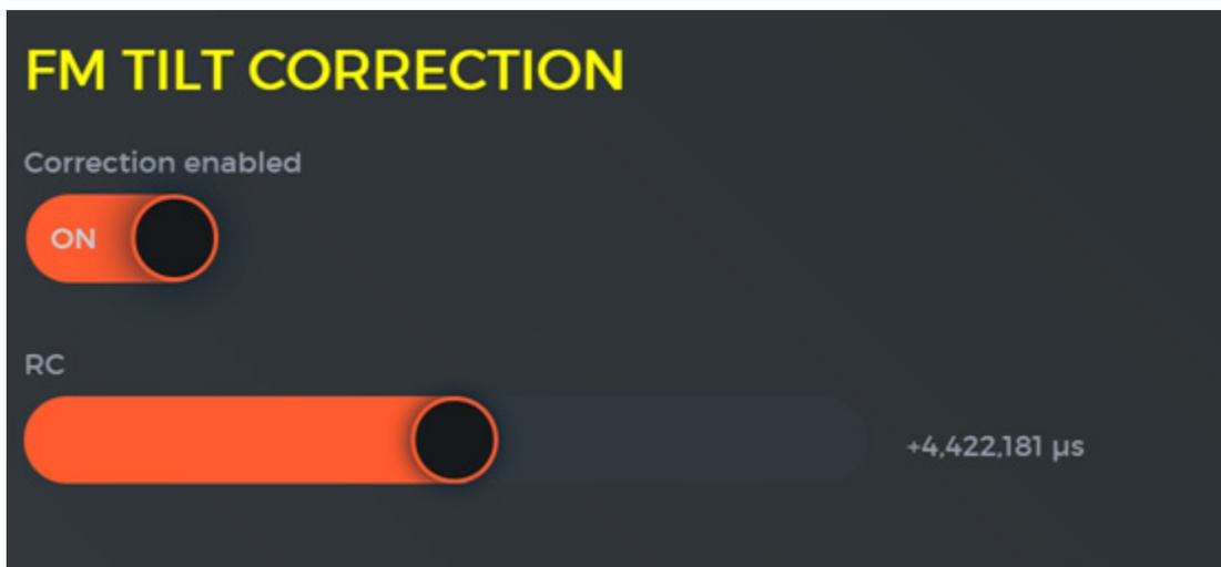
Use these together to compensate for sound cards that are not DC-coupled or might have other non-linearity. To ensure the best results, even sound cards advertised as DC-coupled should be checked for non-linearity before being fed into a transmitter.
